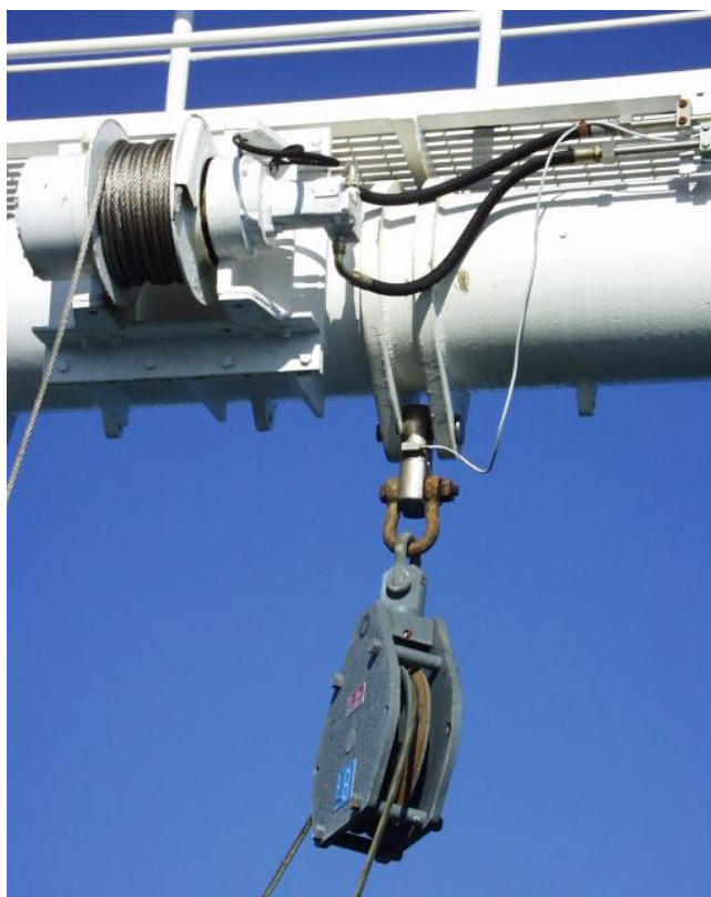
Figure 1: The T20 AEP load cell on the OGS-Explora A-frame.
